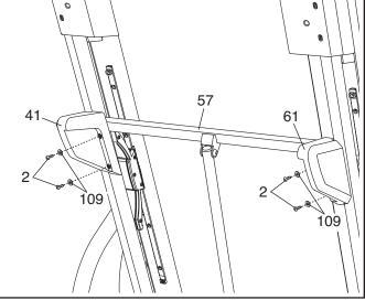
18. Make sure that all parts are properly tightened before you use the treadmill. If there are sheets of plastic on the treadmill decals, remove the plastic. To protect the floor or carpet, place a mat under the treadmill. Note: Extra hardware may be included. Keep the included hex key in a secure place; the hex key is used to adjust the walking belt (see pages 27 and 28).
